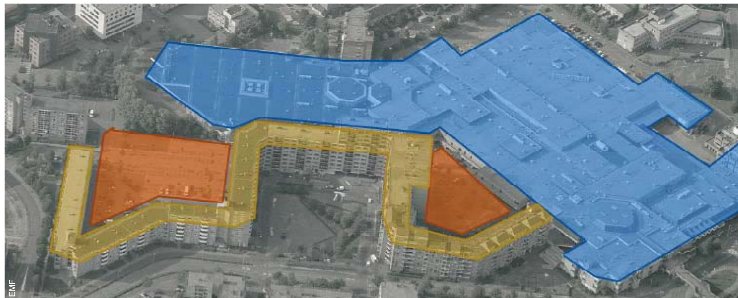
In the Southern part of Arnhem the shopping centre Kronenburg and the surrounding residential neighbourhood are a “climatic hot spot”: Long buildings block ventilation, parking without shading, lack of green space in residential area, high roof temperatures on shopping centre in summer.
