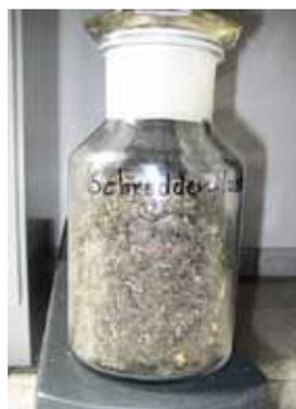
Material from scrapped cars replacing black coal to reduce the use of fossil energy.
