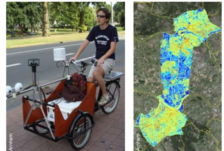
*Analysing the city climate with special bicycles and the heat scan in parts of the City Region Arnhem Nijmegen.*
