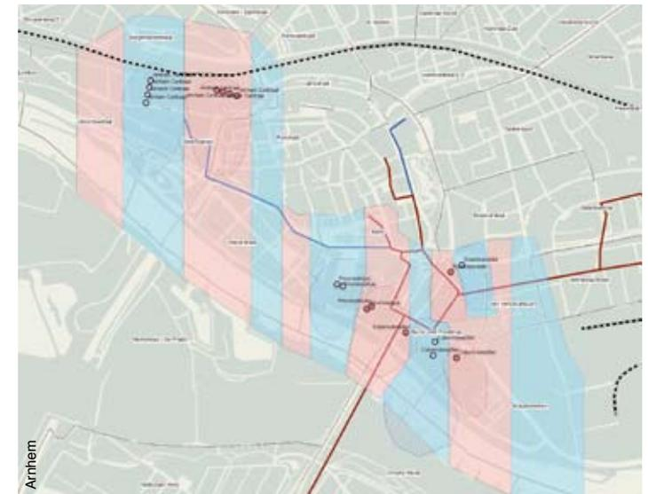
*The masterplan for cold-heat-storage – light blue zones for cold and light red zones for heat storage – for the inner city of Arnhem shall allow to make best use of the available capacity.*
