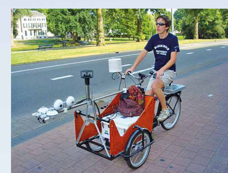
Analysing the city climate of the City Region Arnhem-Nijmegen (The Netherlands) with special bicycles
